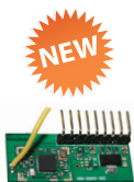
CM-RX-DBK Kinetic™ plug-in no-battery wireless daughterboards for CM-RX-91 or CM-RX-92 V2 receivers
