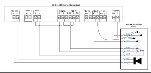
CX-DESPK is supplied with a stainless-steel faceplate that can be easily mounted to a single gang electrical box. Only 9/18" depth is required!
